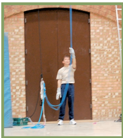
Fig 5 Fixed rope system in use, the person lunging takes up the slack in the rope, but if anything goes wrong the rope is still attached to the floor.
